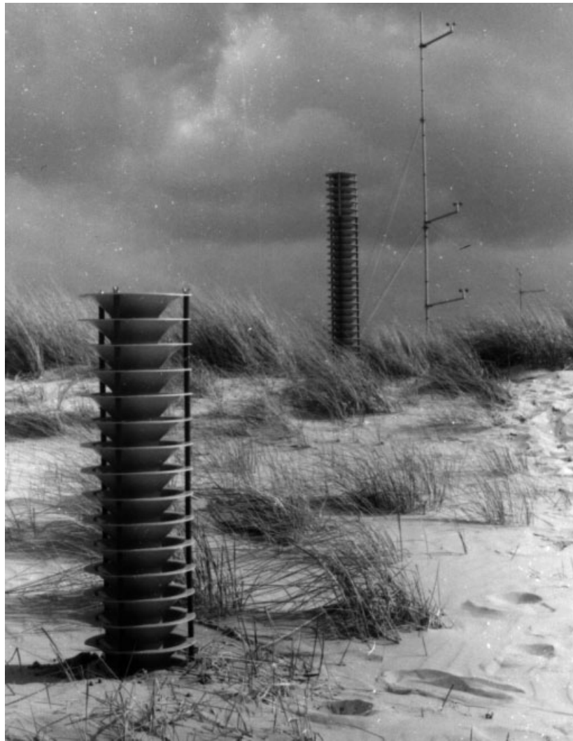
Figure 2. Saltation sand trap. The number of trays can be adapted, according to the height of the sand cloud
